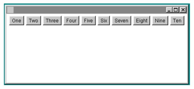
Bear in mind that both images are the display for exactly the same Java code. The only thing that has changed is the width. The FlowLayout manager automatically changes the layout of the components when the Frame is re-sized. If you were to make the Frame very small the FlowLayout manager would change the layout so that the buttons were wrapped around in several rows.
