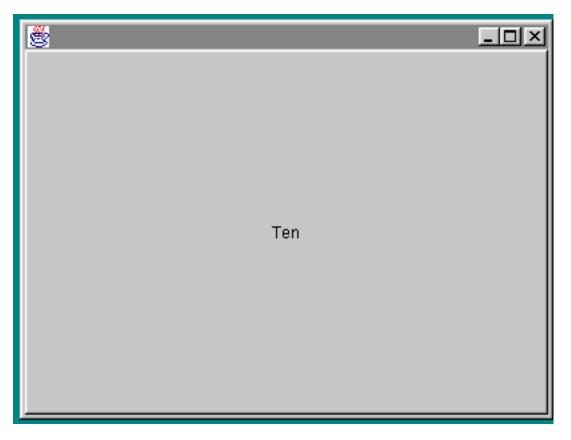
The reason you get this unexpected big button in the center is that the BorderLayout uses a set of coordinates when arranging components. It divides its surface area up into
